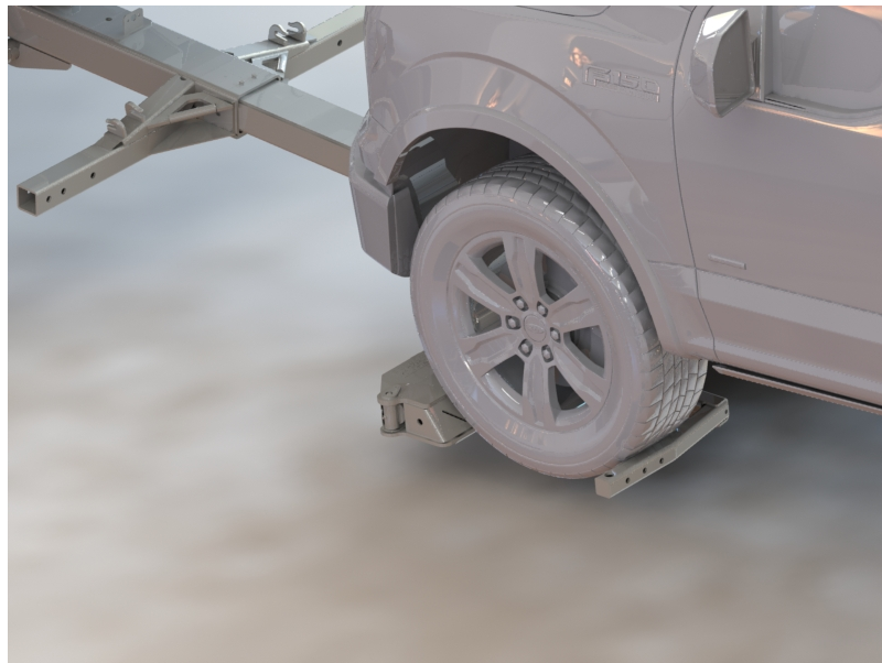
FIGURE 101 – CLAMPING THE L-ARMS AROUND THE WHEELS
