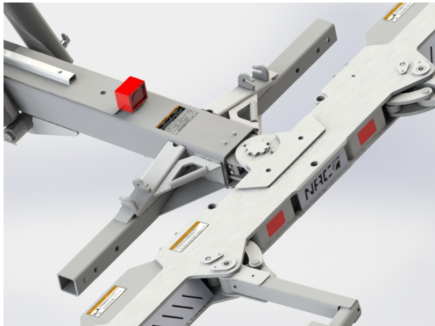
FIGURE 92 – SAFE LOADER CAMERA PLACEMENT ON THE WHEEL LIFT
