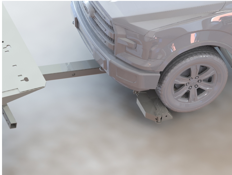
FIGURE 100 – T-BAR MAKING CONTACT WITH THE FRONT WHEELS (CLOSE-UP)
