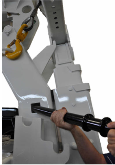
FIGURE 21 – INSERTING THE UNDERLIFT STORAGE PIN (EXAMPLE)
