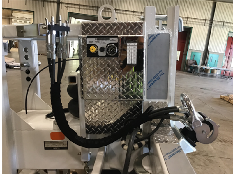
FIGURE 29 – PLACING THE CABLES AND HOSES IN THE DOCKING BRACKET (EXAMPLE)
