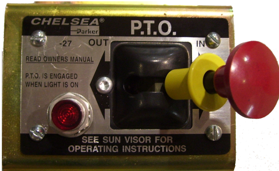
FIGURE 16 – PNEUMATIC PTO CONTROL
