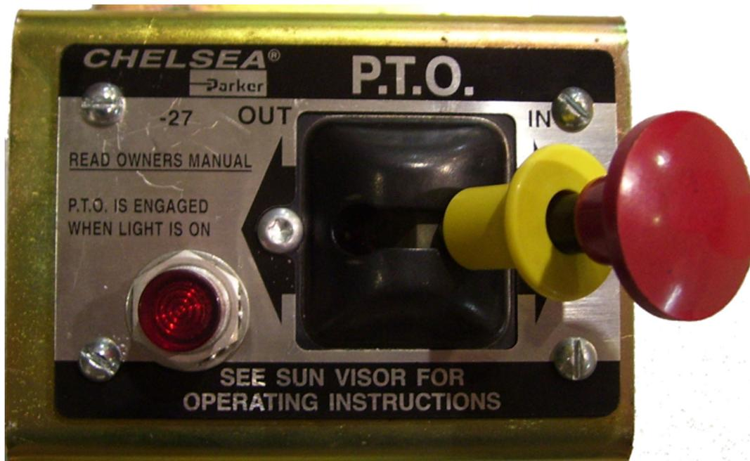
FIGURE 16 – COMMANDE D'UNE PRISE DE FORCE PNEUMATIQUE
