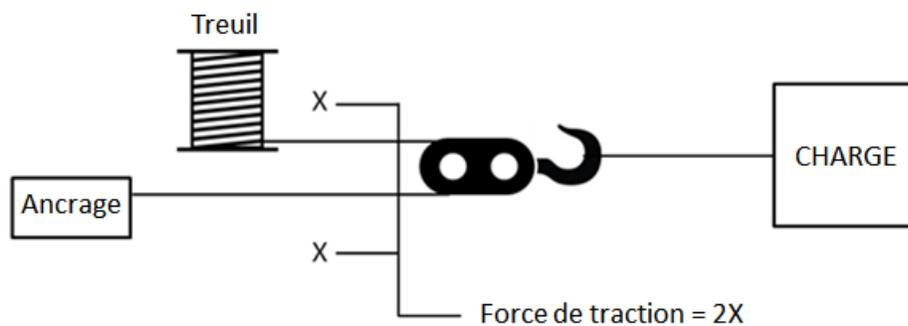
FIGURE 14 – CALCULER L'AUGMENTATION DE CAPACITÉ D'UN TREUIL
