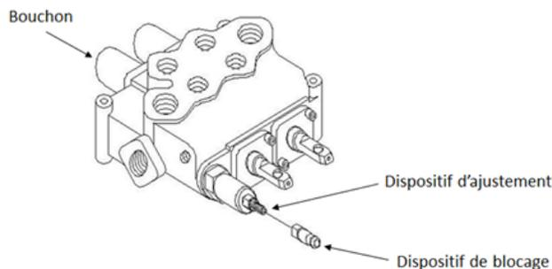
**FIGURE 31 — AJUSTER LA PRESSION HYDRAULIQUE (SOUPAPE DE SURPRESSION PRINCIPALE)**
