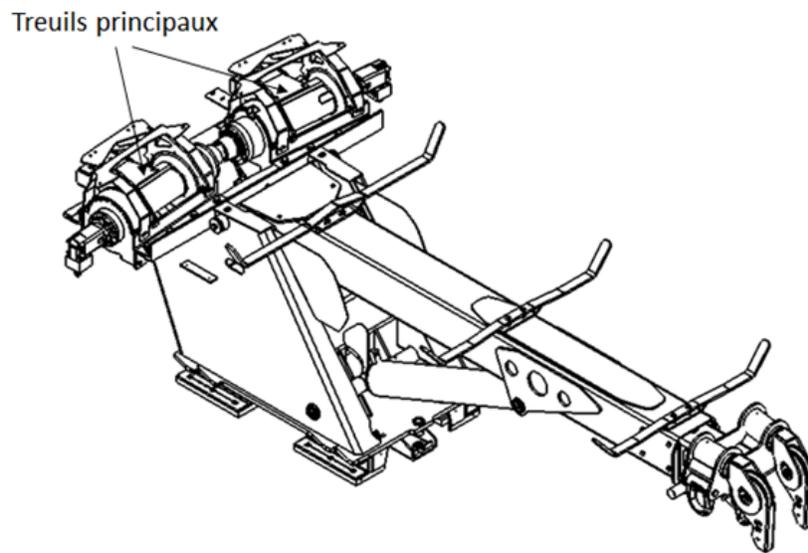
**FIGURE 24 – EMBLACEMENT DES TREUILS**
