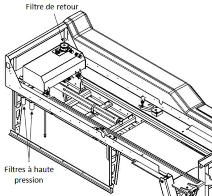
FIGURE 29 – FILTRES – 20CS ET 25CS
