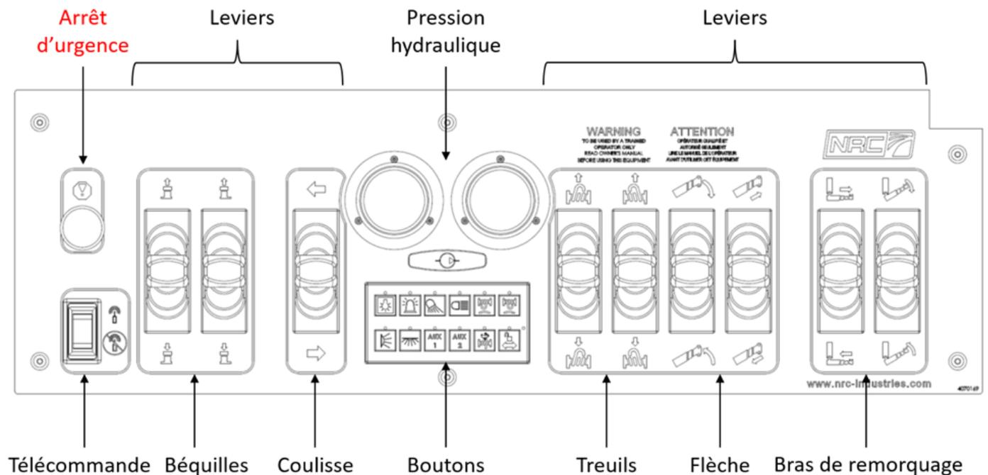
FIGURE 5 – PANNEAU DE COMMANDE CÔTÉ CONDUCTEUR (AVEC LEVIERS ÉLECTRONIQUES OPTIONNELS)
