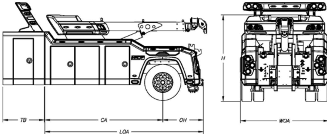
FIGURE 8 – DIMENSIONS DU CHÂSSIS (EXEMPLE)
