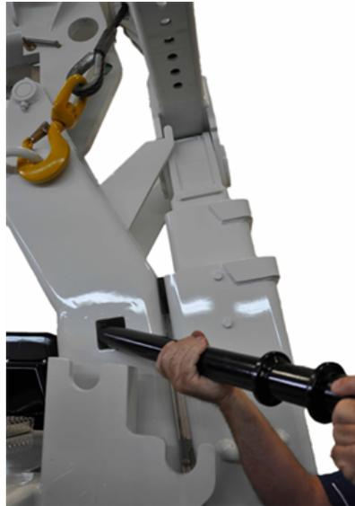
FIGURE 17 – INSÉRER L'AXE DE SUPPORT DU BRAS DE REMORQUAGE (EXEMPLE)
