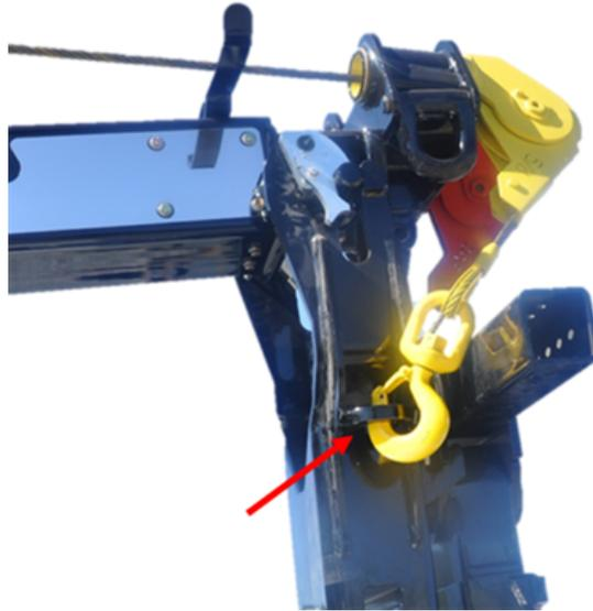
FIGURE 20 — FIXER LES CÂBLES AUX ŒILLETS (EXEMPLE)
