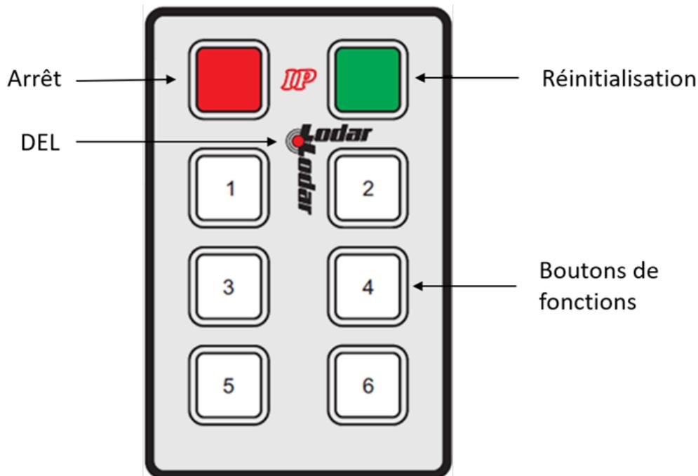
FIGURE 6 – TÉLÉCOMMANDE (À SIX BOUTONS DE FONCTIONS)
