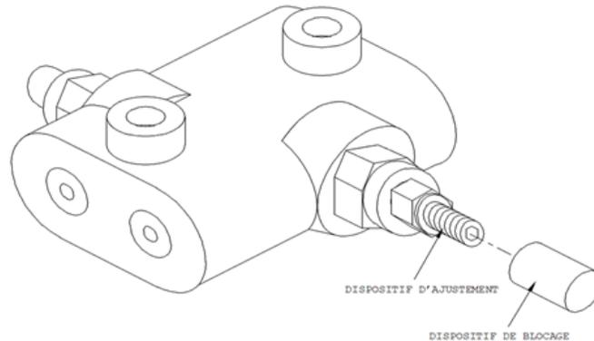
FIGURE 34 – AJUSTEMENT DE LA SOUPAPE D'AMORTISSEMENT
