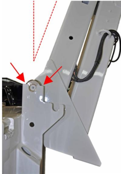
**FIGURE 21 – PLACER LE BRAS DE REMORQUAGE DANS LES RAILS (EXEMPLE)**
