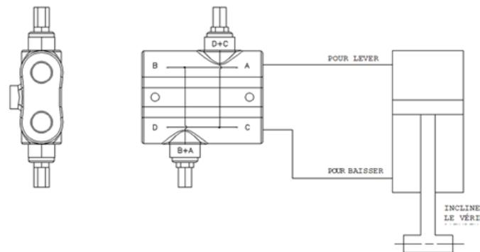
FIGURE 33 – AJUSTEMENT DE LA SOUPAPE D'AMORTISSEMENT DU BRAS DE REMORQUAGE
