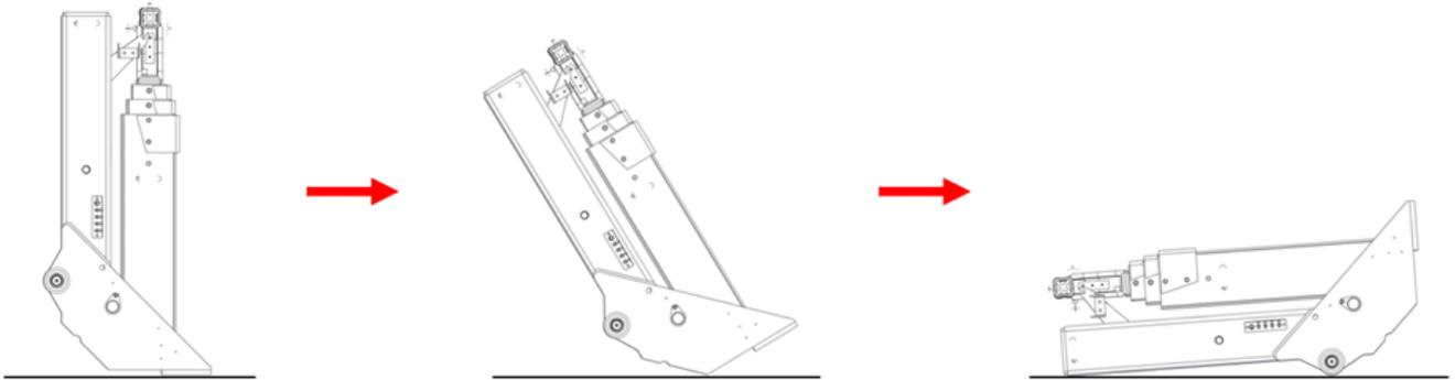
FIGURE 22 – PLACER LE BRAS DE REMORQUAGE SUR UNE SURFACE PLATE (EXEMPLE)
