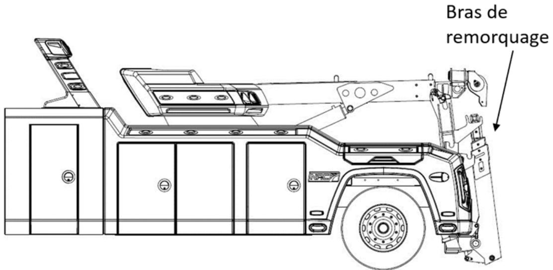
FIGURE 2 – CHÂSSIS AVEC BRAS DE REMORQUAGE (EXEMPLE)
