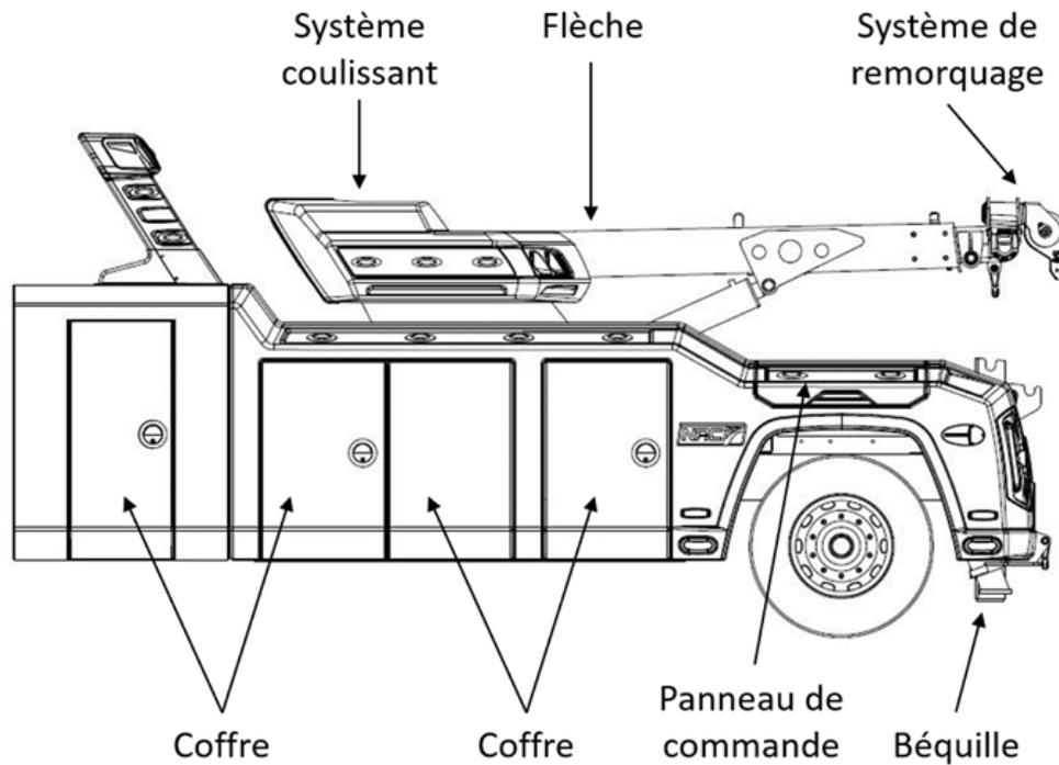
FIGURE 1 – CHÂSSIS SANS BRAS DE REMORQUAGE (EXEMPLE)
