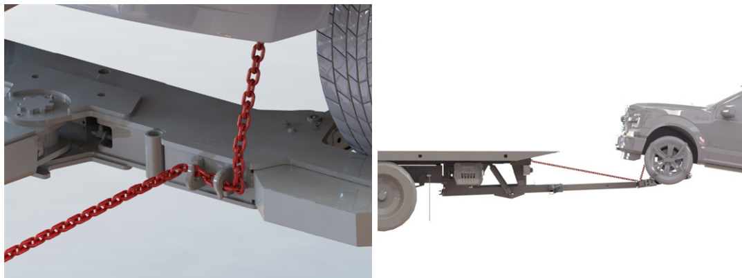
FIGURE 106 – SECURING THE VEHICLE TO THE CARRIER WITH THE SAFETY CHAINS
