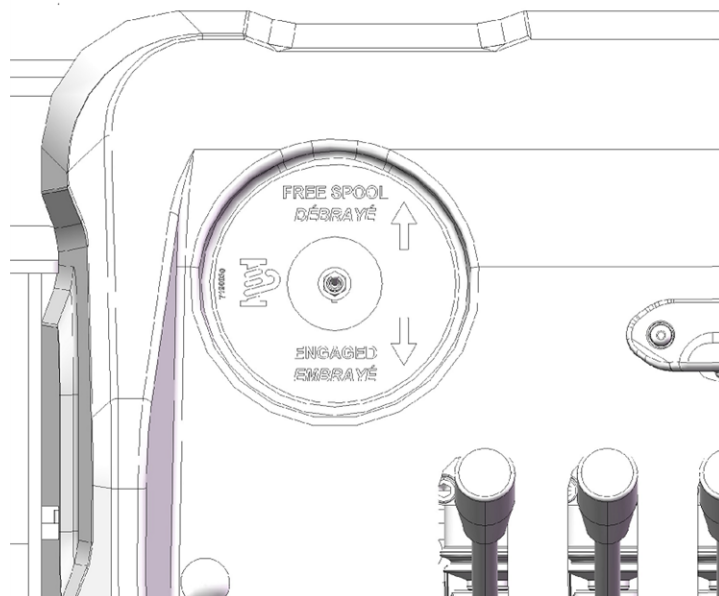
FIGURE 23 – SWITCH USED TO DISENGAGE OR ENGAGE THE WINCH
