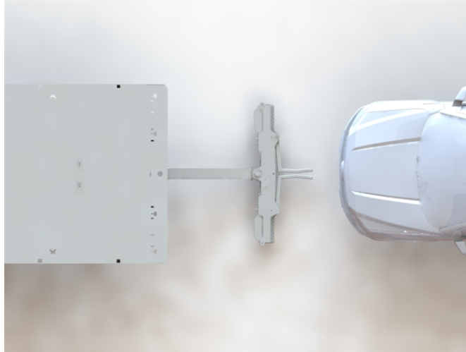
FIGURE 98 – CENTERING THE T-BAR BETWEEN THE FRONT WHEELS
