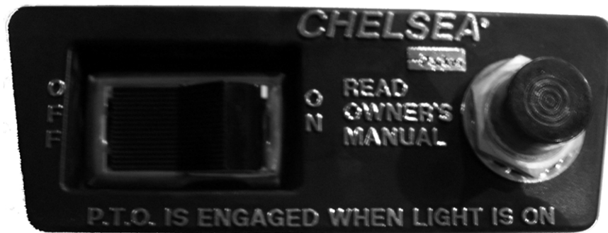
FIGURE 17 – ELECTRIC PTO CONTROL
