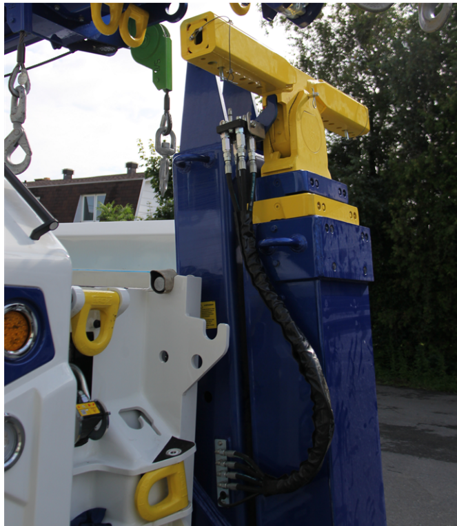
FIGURE 24 – PUT THE HYDRAULIC LINES IN THE DOCKING BRACKET (EXAMPLE)
