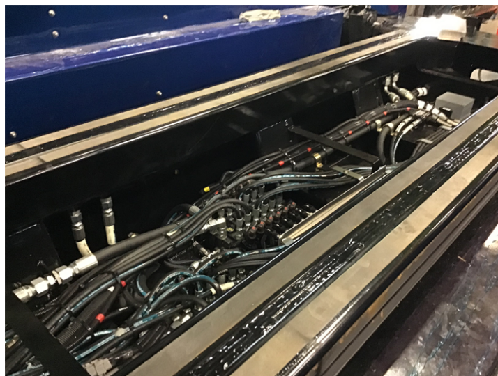
FIGURE 43 – POSITION OF THE VALVES INSIDE THE WRECKER BODY (CSR50 AND CSR65)
