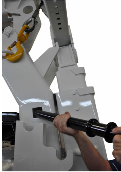
FIGURE 21 – INSERTING THE UNDERLIFT STORAGE PIN (EXAMPLE)
