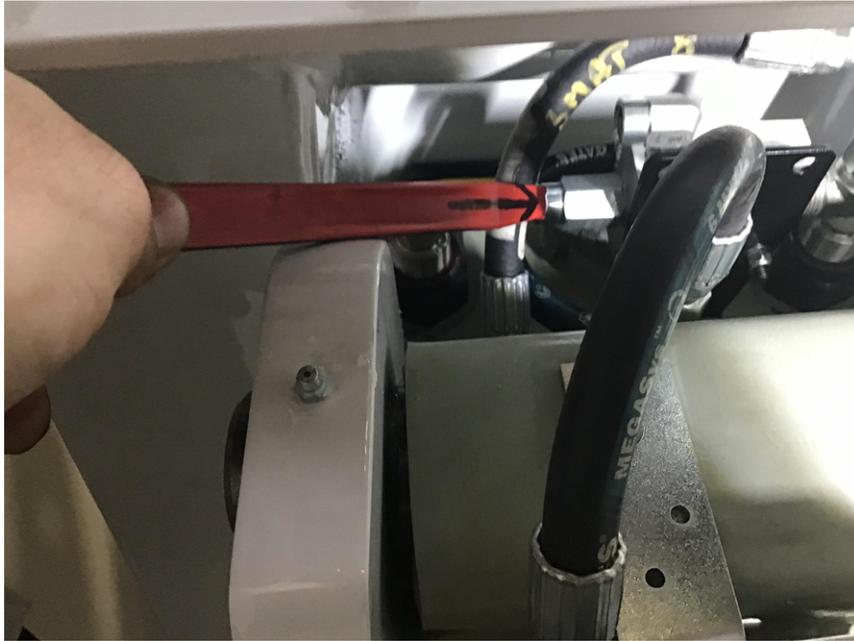
FIGURE 54 – EMBLACEMENT DE LA SOUPAPE DE SÉQUENCE
