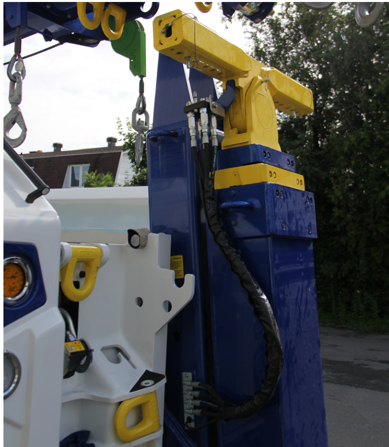
FIGURE 29 – PUT THE HYDRAULIC LINES IN THE DOCKING BRACKET (EXAMPLE)
