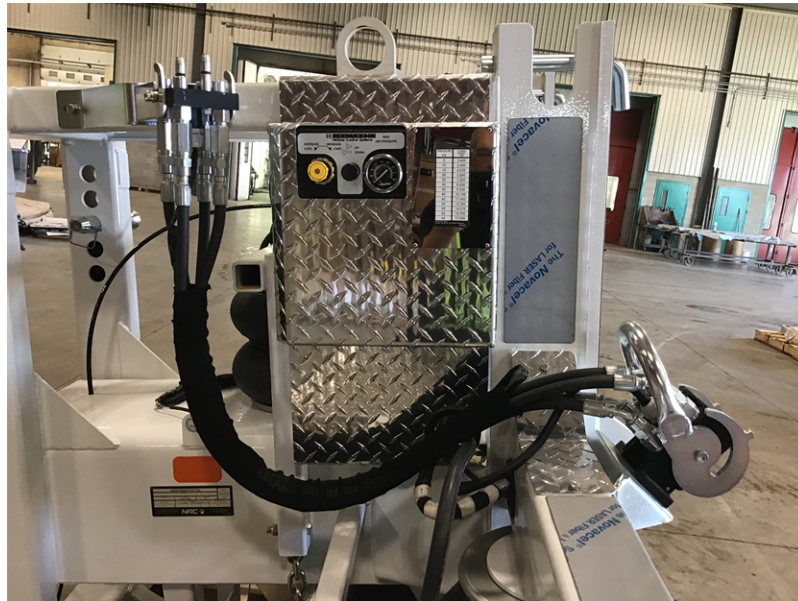
FIGURE 34 – PLACING THE CABLES AND HOSES IN THE DOCKING BRACKET (EXAMPLE)
