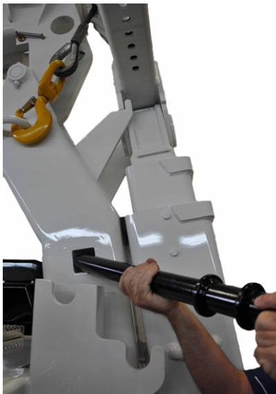
FIGURE 26 – INSERTING THE UNDERLIFT STORAGE PIN (EXAMPLE)
