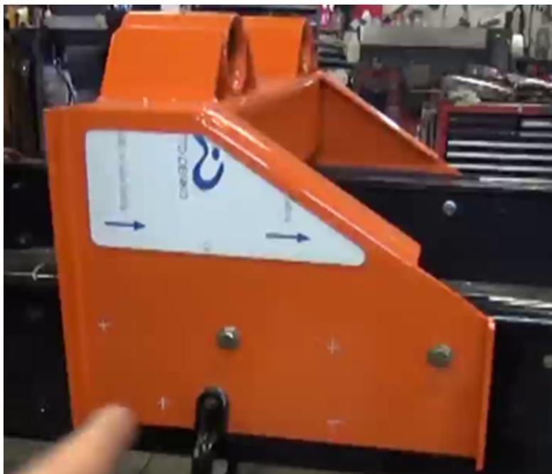
FIGURE 18 – RÉCEPTACLE AVANT FIXÉ AU TRACTEUR
