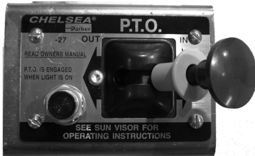
FIGURE 18 – COMMANDE D'UNE PRISE DE FORCE PNEUMATIQUE
